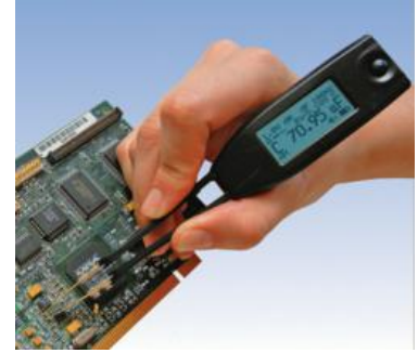
Smart Tweezers LCR-meter simplifies PCB debugging
