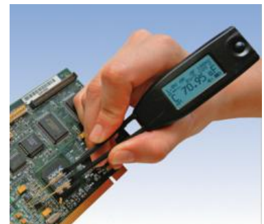
Smart Tweezers LCR-meter simplifies PCB debugging
