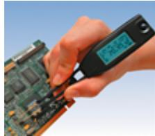
Smart Tweezers LCR-meter simplifies PCB debugging
