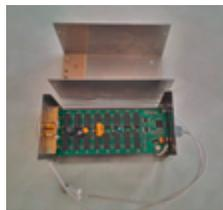
Smart Tweezers and LCR-Reader Calibration Fixture
