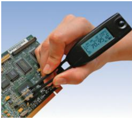
Smart Tweezers LCR-meter simplifies PCB debugging
