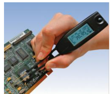
Smart Tweezers LCR-meter simplifies PCB debugging
