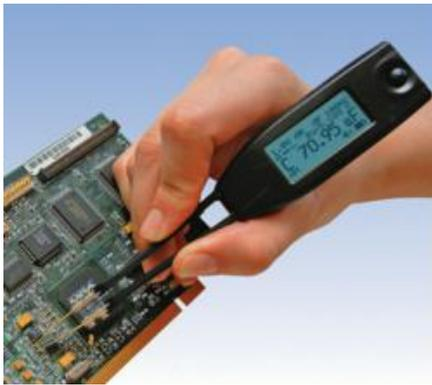
Smart Tweezers LCR-meter simplifies PCB debugging
