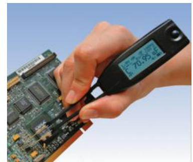
Smart Tweezers LCR-meter simplifies PCB debugging
