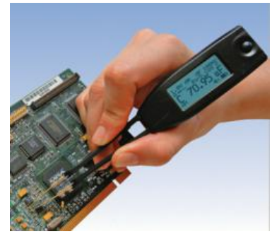
Smart Tweezers LCR-meter simplifies PCB debugging
