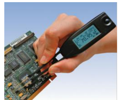
Smart Tweezers LCR-meter simplifies PCB debugging
