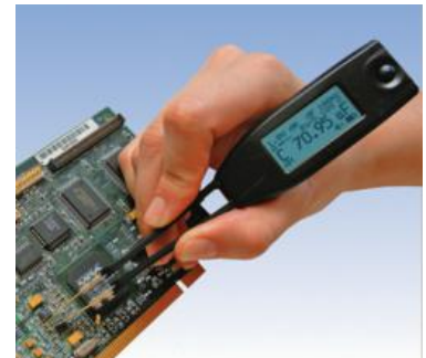
Smart Tweezers LCR-meter simplifies PCB debugging
