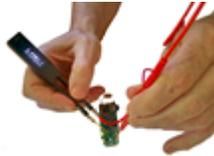
LCR-Reader Probe Connector Kit extends the reach of LCR-Reader's probes
