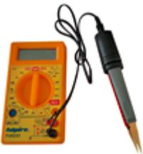
LED Tester Tweezers for easy LED Testing
