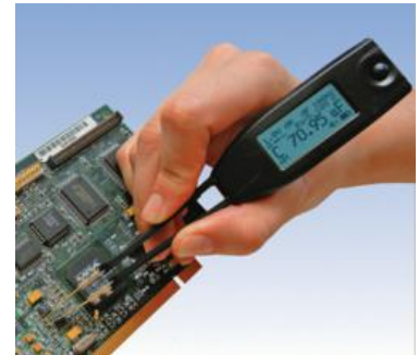
Smart Tweezers LCR-meter simplifies PCB debugging
