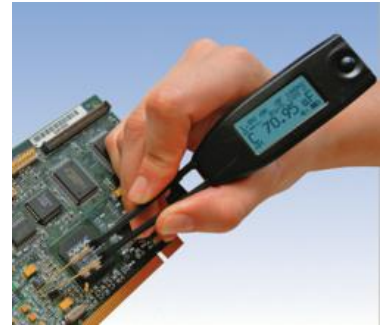
Smart Tweezers LCR-meter simplifies PCB debugging
