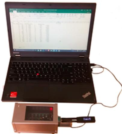
Siborg's new calibration fixture testing an LCR-Reader LCR and ESR meter
