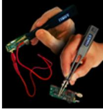
LCR-Reader and LCR-Reader Probe Connector
