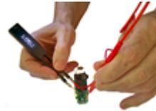
LCR-Reader Probe Connector Kit extends the reach of LCR-Reader's probes
