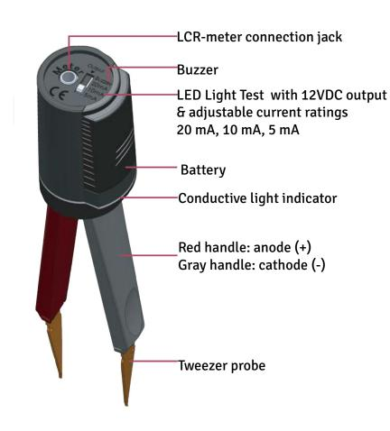
**Warning: Do Not Test Electrified Components**
