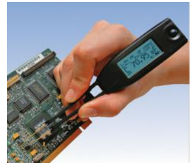
Smart Tweezers LCR-meter simplifies PCB debugging
