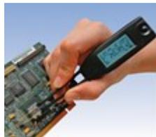
Smart Tweezers LCR-meter simplifies PCB debugging
